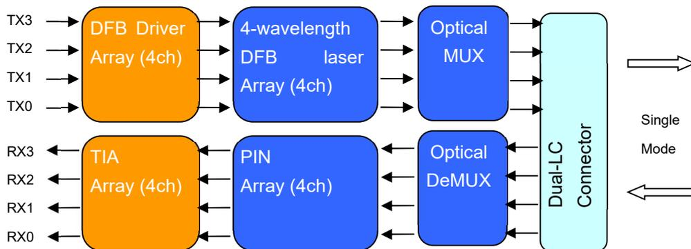
**Figure 1: 40Gb/s QSFP IR4 Transceiver Block Diagram**
