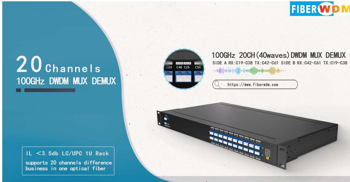
The 20ch(40waves) DWDM MUX/ DEMUX is used in pairs, designed by FIBERWDM, in side A, the waves are: RX C19 to C38(1562.23nm~1546.92nm), TX C42 to C61(1543.73nm~1528.77nm); And in side B, the waves are: RX C42 to C61(1543.73nm~1528.77nm), TX C19 to C38(1562.23nm~1546.92nm).
