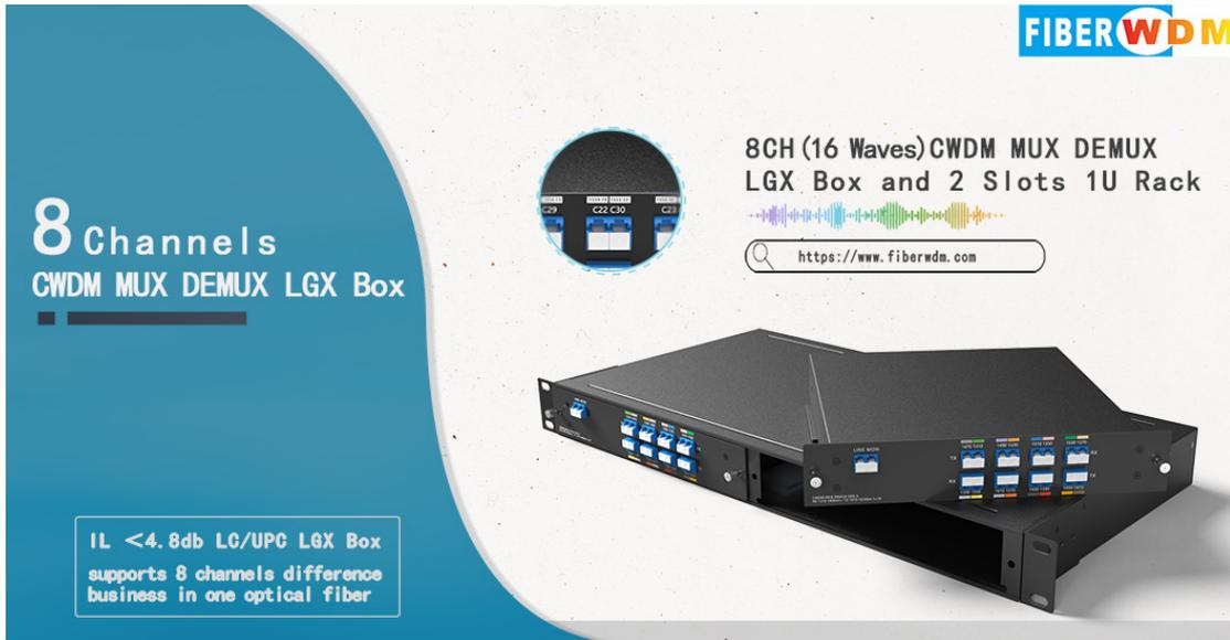
The single fiber 8channels (16 waves) CWDM MUX DEMUX is designed by FIBERWDM, A side's waves are : RX 1310nm to 1450nm/ TX 1470nm to 1610nm, and B side's waves are: RX 1470nm to 1610nm/ TX 1310nm to 1450nm; it is passive CWDM device and plug-in LGX box, can plug in 2slot 1u rack, support 8channels difference business in one optical fiber for bi-direction point-to-point transmission.
