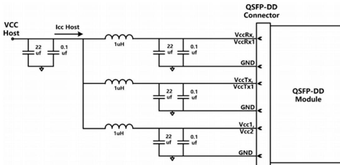
Figure 2. Recommended power supply filter.
