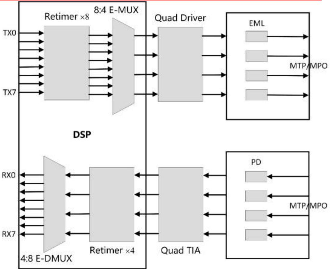
Figure 3. Transceiver block diagram.
